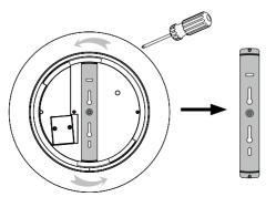
Pull out the bracket anticlockwise by screw driver, take out the bracket.
