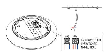
(A) wiring diagram only for NON-emergency function light.
