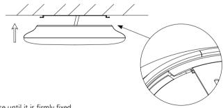
Push the lamp upward and rotate it into bracket. Rotate the lamp clockwise until it is firmly fixed.
