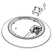
Remove the terminal block cover and crimping clip.
