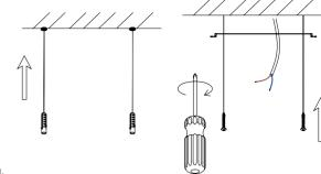
Knock the plastic anchor into ceiling, fix the bracket with screws on the ceiling.
